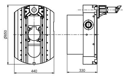
Facing head is mounted manually on the headstock (centring hole of the hollow spindle).
