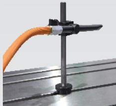
This system cools tools by using coolant, which is externally supplied by a jet.
