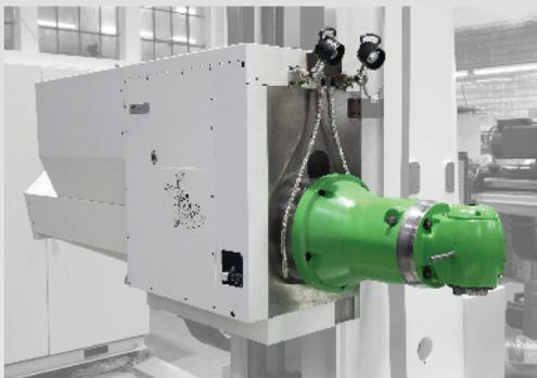
The FP40-10 milling head can be used to mill in planes parallel to the machine's workspindle axis and to bore in planes vertical to the workspindle axis.
