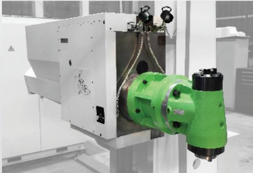
The HPR50 milling head can be used to mill in planes parallel to the machine's workspindle axis and to bore in planes vertical to the workspindle axis.
