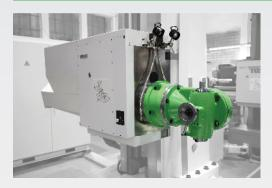
The UFP40-10 universal milling head can be used to mill and bore in arbitrarily inclined planes.
