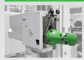
The FP40-10 milling head can be used to mill in planes parallel to the machine's workspindle axis and to bore in planes vertical to the workspindle axis.
