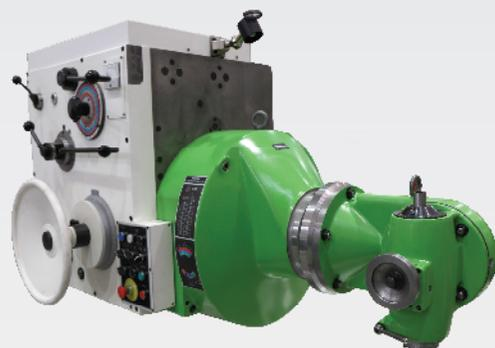
The UFP40-100 universal milling head can be used to mill in various inclined planes parallel to one of the machine's main axes (X, Y, Z) or to bore in the machine's main axes (X, Y, Z).
