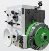
The SP100 spindle clamping support increases the rigidity of the workspindle bearing. Thus, with a fixed spindle stroke in the W axis of over 110 mm, the machining parameters can be raised, while the spindle speed range is reduced.
