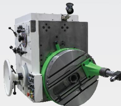
When using the facing head, the TD50 telescopic tool holder allows you to machine deep inner and outer surfaces of larger diameters.
