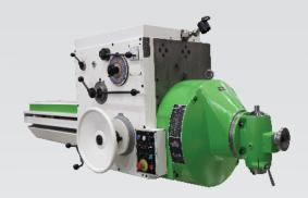
The FP40-100 milling head can be used to mill in the basic and inclined planes parallel to the workspindle axis, or to bore in the basic planes rectangular to the workspindle axis.
