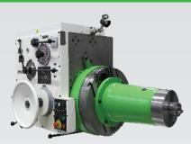
The spindle guiding support considerably increases the rigidity of the workspindle bearing and thus also the number of possible spindle applications, especially for high-power or high-precision machining with larger overhangs – using the full workspindle speed range and stroke.
